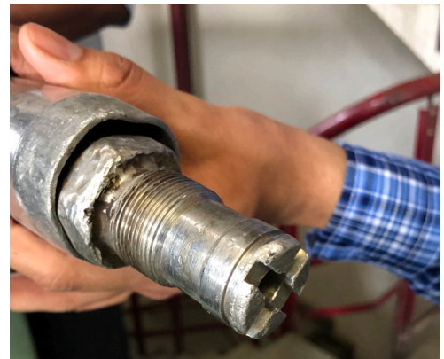
Damage to threads on SDX® III Nozzle.
