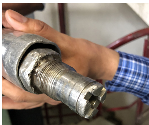
Damage to threads on SDX® III Nozzle.
