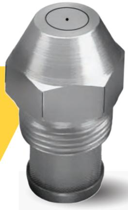
Basic nozzle thread 9/16" – 24 UNEF, with optional adaptors providing 1/8" and 1/4" pipe threads. Flow sizes from 0.5 to 20 with spray angles of 30°, 45°, 60°, 70°, 80°, and 90°.
