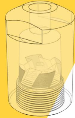
CM 16 – 105 available. One-piece body with removable vane type core. Spray angles of 45° to 110° dependent upon flow size and pressure. See chart for available thread sizes.
